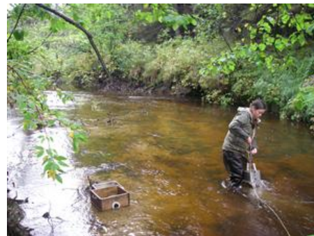
Using an Ekman dredge to collect sediment samples. Source: Hatfield Consultants 2007 (click to enlarge)
