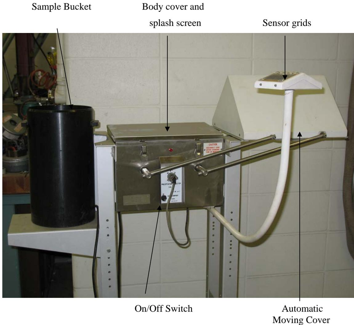
Figure 1.1 Precipitation Collector
